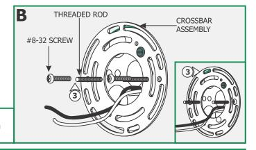
**3:** Mount the crossbar assembly to the electrical box holes with the provided #8-32 screws so that the two threaded rods on crossbar are leveled horizontally.
