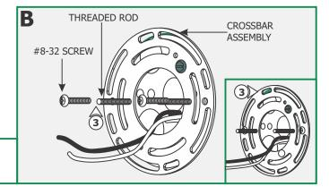
**3:** Mount the crossbar assembly to the electrical box holes with the provided #8-32 screws so that the two threaded rods on crossbar are leveled horizontally.
