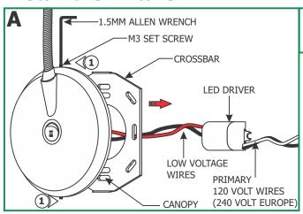
2: Line up the crossbar slots with the electrical box holes, and secure it in place by tightening the two #8-32 screws provided.
