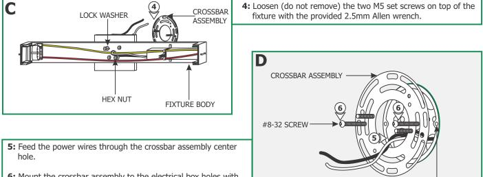
**6:** Mount the crossbar assembly to the electrical box holes with the provided two #8-32 screws.
