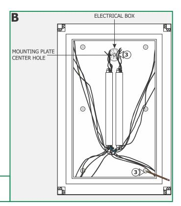
**3:** Align the mounting plate center hole with the electrical box. Level the mounting plate horizontally and mark the six mounting plate holes onto the wall.
