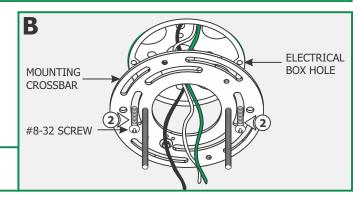
**2:** Install the mounting crossbar to the electrical box holes with the two provided #8-32 screws
