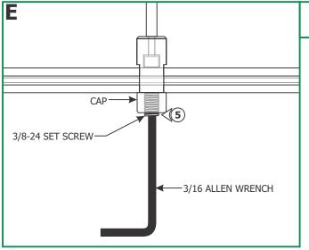
**5:** Tighten the 3/8-24 set screw on the cap firmly with the 3/16 Allen wrench provided for proper power connection.
