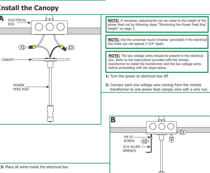
4: Secure the power feed canopy to the electrical box by tightening the two provided #8-32 screws with the 3/32 Allen wrench.
