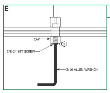
**5:** Tighten the 3/8-24 set screw on the cap firmly with the 3/16 Allen wrench provided for proper power connection.
