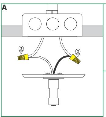
**NOTE:** Use the universal round crossbar (provided) if the electrical box holes are not spaced 2-3/4" apart.
