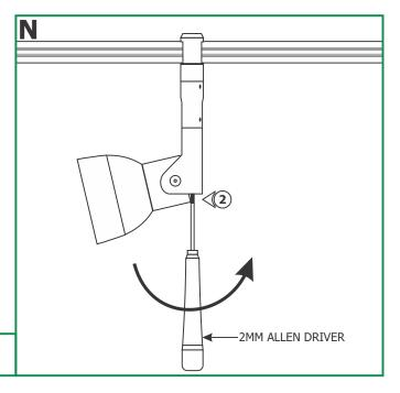
**2:** Use the 2mm Allen driver on the bottom of the Neo arm to tilt the head up or down.
