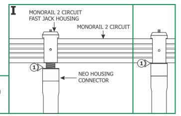
2: Place the Monorail 2 Circuit Fast Jack housing onto the Monorail 2 Circuit and use fingers to tighten the Neo housing connector to the Fast Jack housing. <a href="Make sure that the Neo housing connector">Make sure that the Neo housing connector</a> is not cross threaded.
