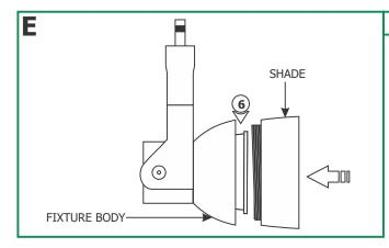
**6:** Tighten the shade completely to fixture body.
