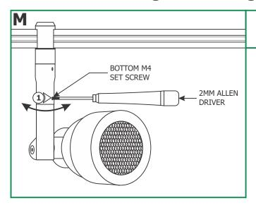
**1:** Rotate the Neo to the desired location and lock the position by tightening the bottom M4 set screw with the 2mm Allen driver.
