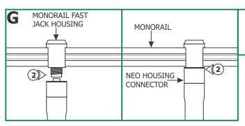
2: Place the Monorail Fast Jack housing onto the Monorail and use fingers to tighten the Neo housing connector to the Fast Jack housing. Make sure that the Neo housing connector is not cross threaded.
