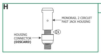
**1:** Remove the Monorail 2 Circuit housing connector from the Monorail 2 Circuit Fast Jack housing and discard it.
