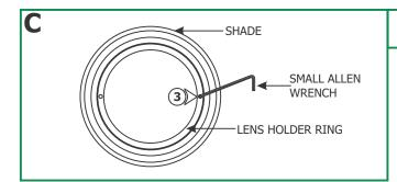
**3:** From the inside of the shade, use a small Allen wrench or a pen point to loosen and remove the lens holder ring.
