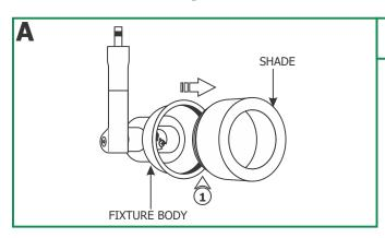
**1:** Loosen and remove the shade completely out of the fixture body.
