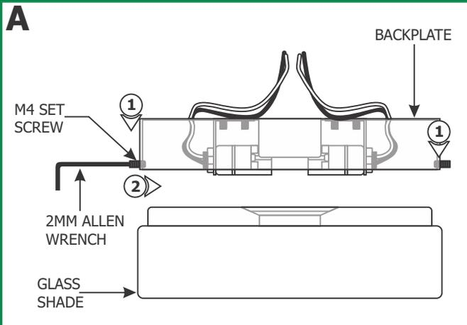
**1:** Loosen the two M4 set screws (**DO NOT REMOVE**) on the backplate with the 2MM Allen wrench provided.
