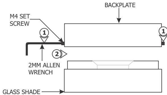
**1:** Loosen the two M4 set screws (**DO NOT REMOVE**) on the backplate with the 2mm Allen wrench provided.
