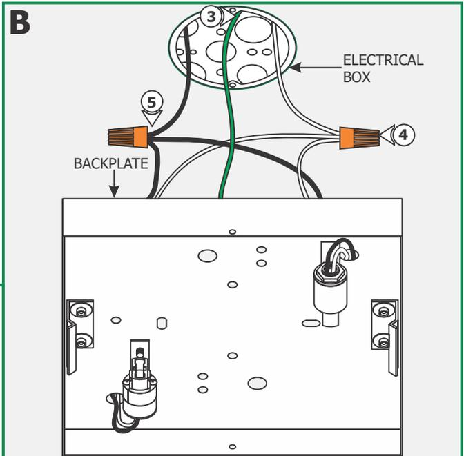
**3:** Make sure that the fixture is grounded in accordance with local electrical codes.
