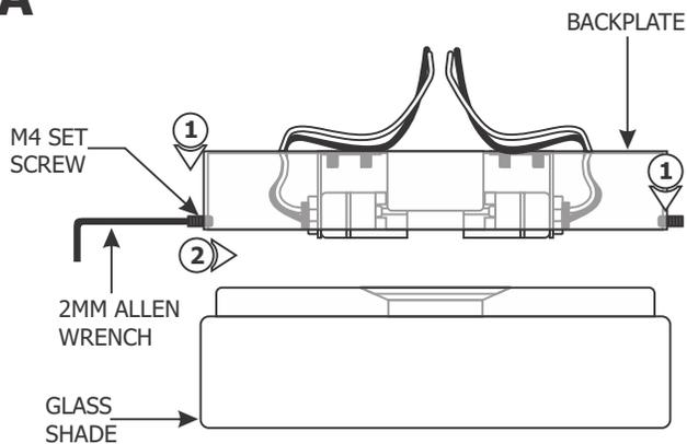
**1:** Loosen the two M4 set screws (**DO NOT REMOVE**) on the backplate with the 2MM Allen wrench provided.
