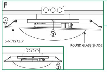
2: Place the edge of the round glass shade into two adjacent spring clips. Slightly push the glass shade against these two spring clips and simultaneously slide the other edge into the other two spring clips. <u>Make sure that the round glass</u> shade sits properly into the four spring clips.
