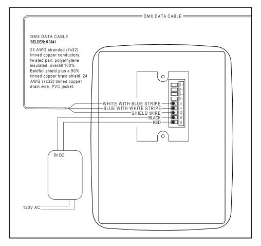
Mount controller to a single gang switch box or two gang electrical junction box.
