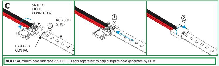
1: Align the +24VDC marking on the soft strip with the black wires of the Snap & Light connector. Insert the exposed contact at the end of the RGB strip under the Snap & Light contacts ensuring that the strip contacts are aligned and covered under the connector contacts.
