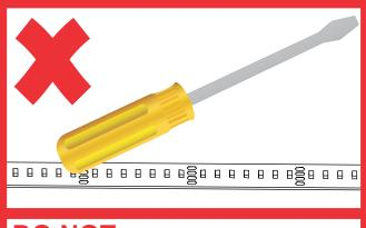
**DO NOT** use any tool to install soft strip to a surface. This will damage the soft strip component.
