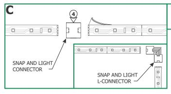
4: Join additional sections of soft strip using Snap and Light straight or directional connectors. Refer to Snap and Light installation instructions.
