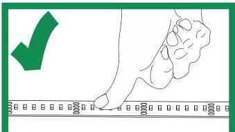
**DO** only ever use fingers to gently install soft strip to a surface **AFTER** cleaning the surface with alcohol.
