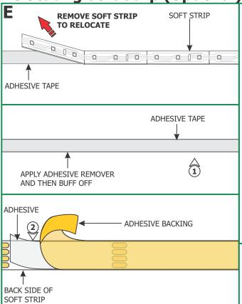
**NOTE:** If relocating the installed soft strip, make sure that the adhesive tape on back of the soft strip covers the entire strip. The adhesive tape isolates the strip from the installation surface. Damaged or inconsistent adhesive tape may cause the contacts on the back of the strip to come in contact with the conductive heat sink which will cause the strip to short and burn. Call Edge Lighting to get replacement adhesive tape and/or optional aluminum heat sink tape (SS-HR-F)
