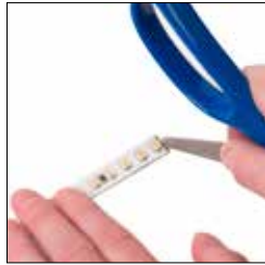
Scrape protective coating from contacts
