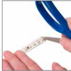
Scrape protective coating from contacts
