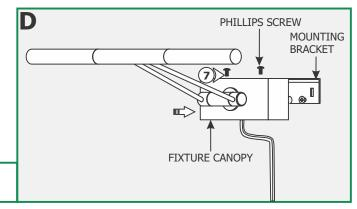
**7:** Place the fixture canopy onto the mounting bracket and tighten the two Phillips screws to secure the fixture in place.
