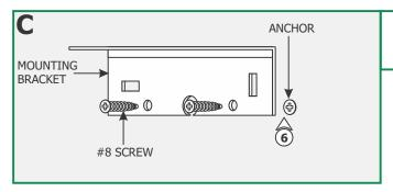
**6:** Line up the mounting bracket holes with the anchors and secure the fixture to the anchors with the two #8 screws provided.
