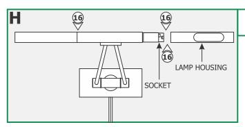
**16:** Pull out the two lamp housings from the fixture to expose the two sockets.
