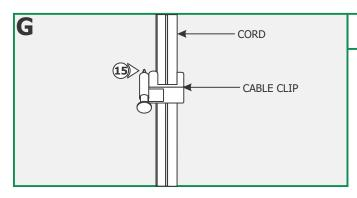
**15:** Use the provided cable clips to secure the cord to the wall, or use a cable cover (not provided).
