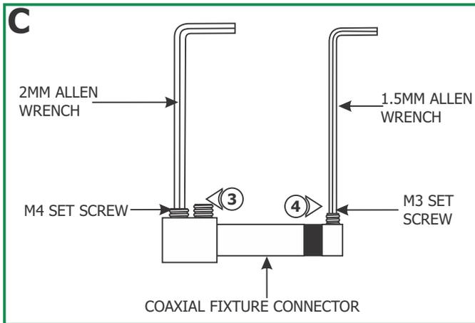
**3:** Loosen the two M4 set screw on base of the coaxial fixture connector with the 2mm Allen wrench provided. **Do not remove these set screws.**
