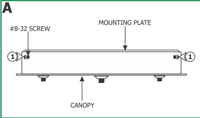
**1:** Loosen and remove the three #8-32 screws from the canopy to remove the mounting plate.
