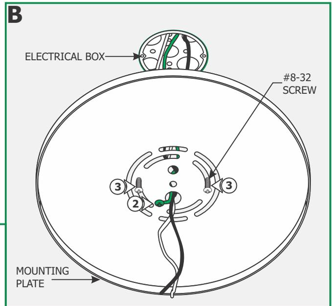
**2:** Make sure the mounting plate is grounded in accordance with local electrical codes.
