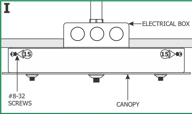
**14:** Place all the wires and wire nut connections inside the canopy.
