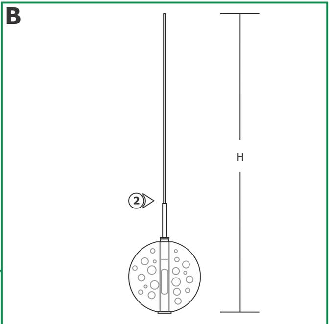
**2:** Cut the coaxial cable to the desired height (H) with a sharp cutter. The overall fixture height is measured from the bottom of the glass shade to the end of the coaxial cable.
