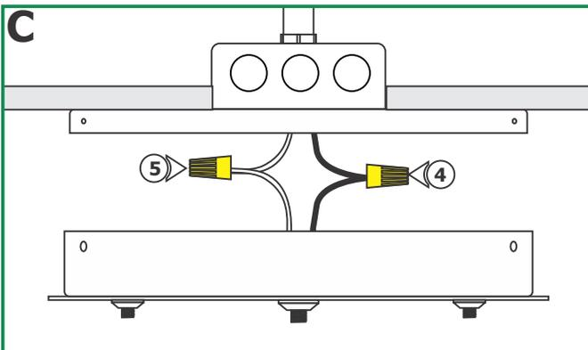
**4:** Connect the white fixture wire to the neutral power wire with a wire nut.
