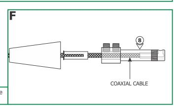
**8:** Feed the coaxial cable into the coaxial fixture connector. The coaxial cable will come to a stop point.
