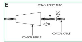
7: Feed the coaxial cable through the conical nipple and flared side of the strain relief tube. Slide the conical nipple and strain relief tube down the coaxial cable.
