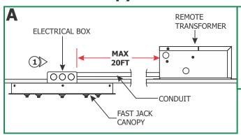
1: Run the low voltage wires from a remote transformer to electrical box where Fast Jack canopy is going to be installed. It is recommended to install the remote transformer near the electrical box to avoid voltage drop. Refer to the instructions provided with remote transformer for low voltage wire size chart. Refer to the low voltage wire size chart provided with the remote transformer.
