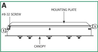
**1:** Loosen and remove the six #8-32 screws around the canopy to remove the mounting plate.
