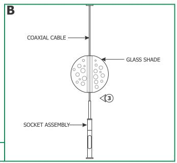
**3:** Feed the coaxial cable through the glass shade, and rest the glass shade over the socket assembly.
