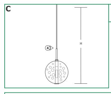
**4:** Cut the coaxial cable to the desired height (H) with a sharp cutter. The overall fixture height is measured from the bottom of the glass shade to the end of the coaxial cable.
