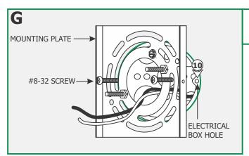
**10:** Mount the mounting plate to the electrical box holes with the provided two #8-32 screws.
