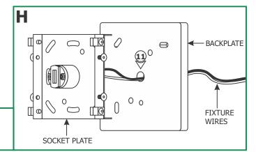
**11:** Feed the fixture wires from the socket plate into the backplate center hole.
