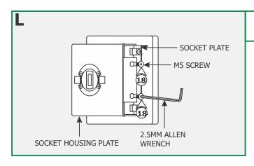
**18:** Push the socket housing plate slots onto the M5 screws and tighten them with the 2.5mm Allen wrench.
