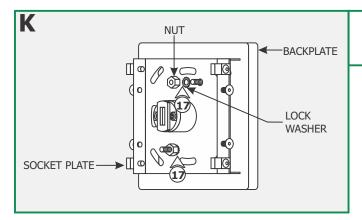
**17:** Replace and tighten the two lock washers and nuts to secure the socket plate onto the backplate.
