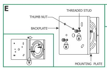
**8:** Remove the two thumb nuts from the backplate threaded studs.
