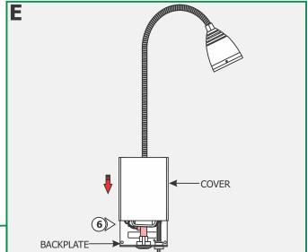
**6:** Replace and slide the cover down completely onto the backplate.
