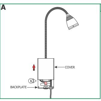
1: Remove the cover by sliding it up and then off the backplate.
