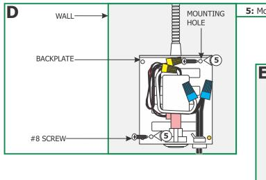
**5:** Mount the backplate to the anchors with the two #8 screws.
