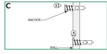
**NOTE:** Omit steps 3 to 5 if installing the fixture onto a surface other than drywall like bedroom wood board. Use the provided screws to mount the backplate directly to the wood board.
