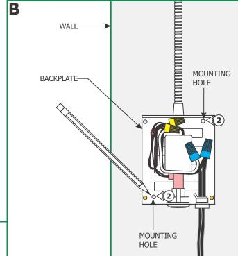
2: Hold the backplate against the surface where the fixture is going to be mounted. Level the backplate vertically and mark the two mounting holes on the surface.
