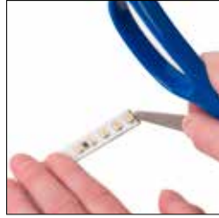
Scrape protective coating from contacts
