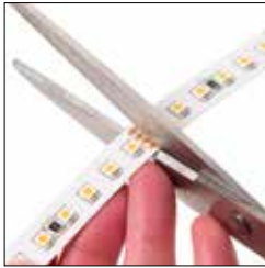
Cut in middle of joining contacts
