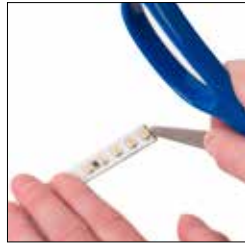
Scrape protective coating from contacts
