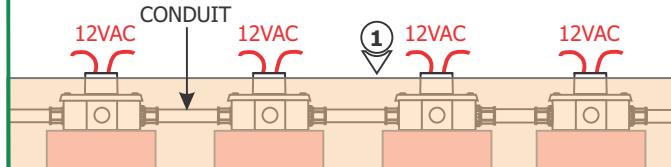
**1:** Align and secure the each trim housing to the octagon electrical box holes with the two #8-32 screws (not provided).
