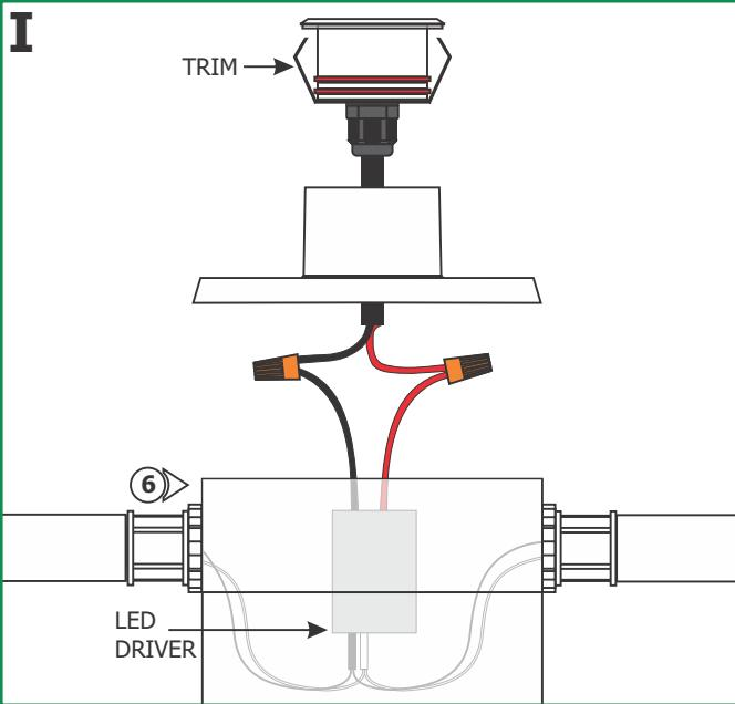
**NOTE:** For outdoor installation, use water proof outdoor wire nuts for power connection.
