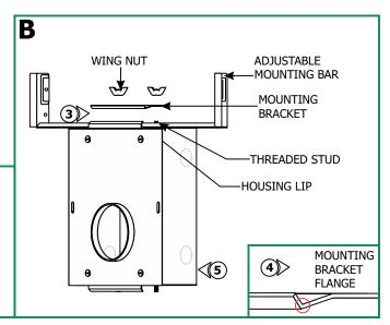
**NOTE:** The adjustable mounting bars mount to joists (studs) that are spaced 16" to 24" apart.
