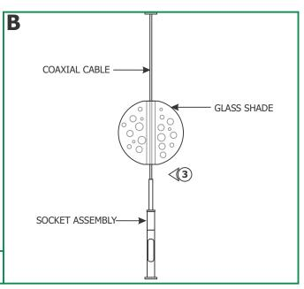
**3:** Feed the coaxial cable through the glass shade, and rest the glass shade over the socket assembly.
