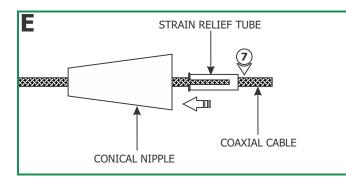
**7:** Feed the coaxial cable through the conical nipple and flared side of the strain relief tube. Slide the conical nipple and strain relief tube down the coaxial cable.
