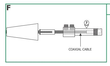
**7:** Feed the coaxial cable into the coaxial fixture connector. The coaxial cable will come to a stop point.
