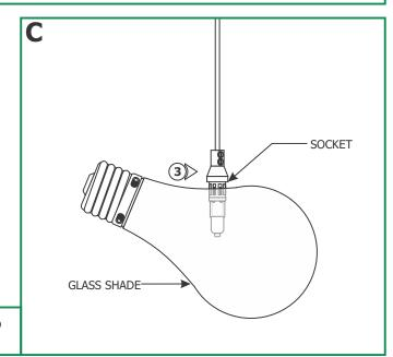
**3:** Push the socket assembly back into the glass shade hole to secure in place.
