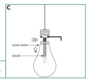
**3:** Align the socket assembly set screws to the glass shade hole. While holding the glass shade in place, secure it by tightening the three M4 set screws with the provided 2mm Allen wrench.
