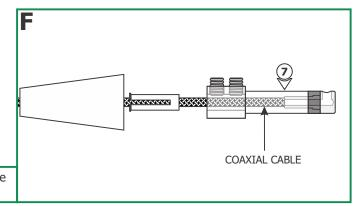
**7:** Feed the coaxial cable into the coaxial fixture connector. The coaxial cable will come to a stop point.
