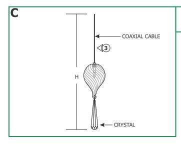
**3:** Cut the coaxial cable to the desired length (H) with a sharp cutter. The overall fixture height is measured from the bottom of the glass shade to the end of the coaxial cable.
