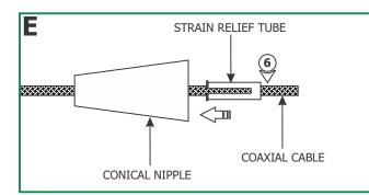
**6:** Feed the coaxial cable through the conical nipple and flared side of the strain relief tube. Slide the conical nipple and strain relief tube down the coaxial cable.
