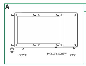
**1:** Loosen the six Phillips screws on front of the power supply to remove the cover.
