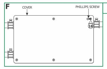
**18:** Replace the power supply cover and secure it by tightening the six Phillips screws.
