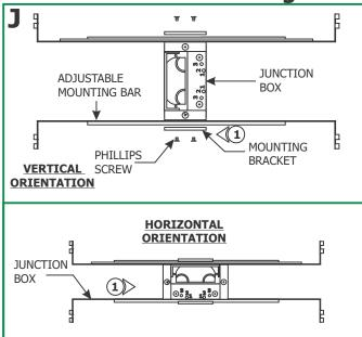
1: Mount each adjustable mounting bar to one side of the junction box (mounts to any side of the housing depending on the orientation of the channel) and secure them with the mounting brackets and two Phillips screws provided.
