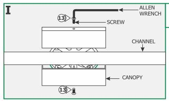
**13:** Place each canopy piece against the channel & line up the canopy hole with the crossbar hole. Secure the canopy in place with the screw & Allen wrench provided.
