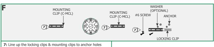
7: Line up the locking clips & mounting clips to anchor holes and secure them by tightening the two #6 screws through the clip holes followed by the washers into the anchors.
