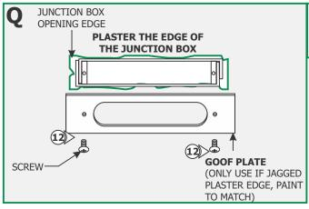
**12: Optional:** Use the Goof Plate if the junction box opening has a lot of imperfection/jagged edges. Install the provided goof plate (paint to match prior) with the two screws.
