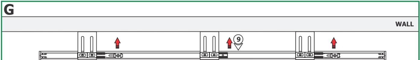
**9:** Channel can be adjusted towards or away from the wall up to 2" as desired.
