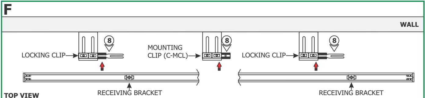
**8:** Align the channel with locking/mounting clips. Carefully snap channel onto the locking/mounting clips then slide 2" into receiving bracket to lock in place.
