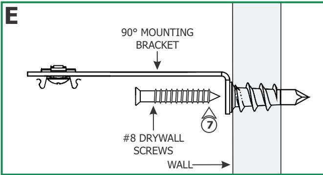
**7:** Install the assembled brackets to the drywall anchors with the provided #8 drywall screws.
