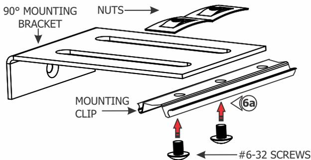
**6b: FOR LOCKING CLIPS,** place inside and align the holes of the locking clip with the mounting clip using the provided #6-32 screws and nuts.
