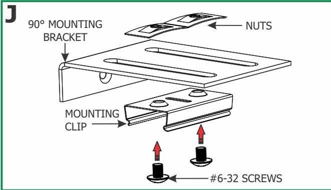
**NOTE:** Install one 90° mounting bracket for each mounting provided with Light Channel.
