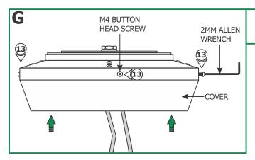
**13:** Replace the cover and tighten the five M4 button head screw around the transformer cover with the provided 2mm Allen wrench.
