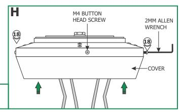
**18:** Replace the cover and tighten the five M4 button head screws around the transformer cover with the provided 2mm Allen wrench.
