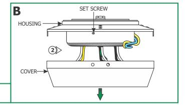
**2:** Unhook the transformer cover from the set screw and remove it from the transformer housing.
