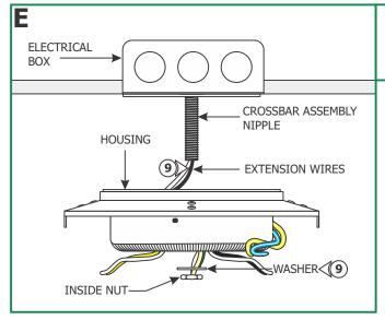
**9:** Feed the extension wires through the transformer housing center hole. Slide the transformer housing onto the crossbar assembly nipple and secure it in place by tightening the washer and inside nut.
