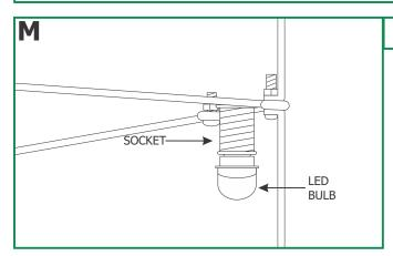
16: Install LED bulbs into each socket
