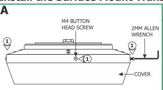
**1:** Loosen and remove the five M4 button head screws around the transformer cover with the provided 2mm Allen wrench.
