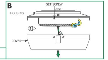
**2:** Unhook the transformer cover from the set screw and remove it from the transformer housing.
