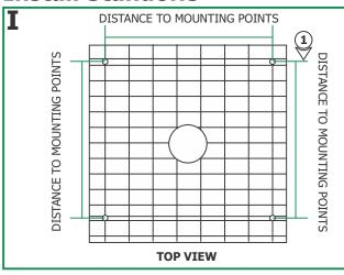
**1:** Measure the distance between the mounting points of the fixture.
