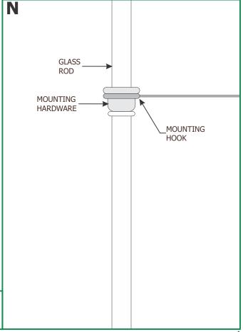
**17:** Carefully install the glass rods by seating them into the mounting hooks. Ensure the mounting hardware is fully seated in the mounting hooks.
