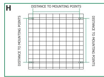
**1:** Measure the distance between the mounting points of the fixture.
