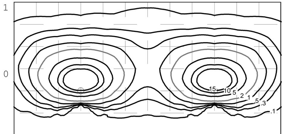
Mouse Lite 20 watt G4 Bi-Pin lamp - Lens height 400mm (15¾")
