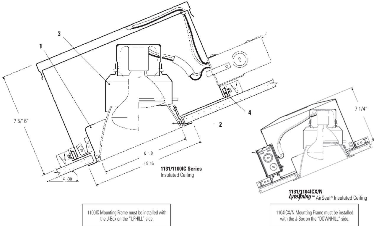
1100IC Mounting Frame must be installed with the J-Box on the "UPHILL" side.
