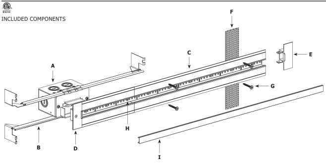
**A. Junction Box:** Mounts behind drywall with Adjustable Mounting Bars. Low voltage 24VDC wires from remote power supply connect to LED wires inside box. Junction Box opening is covered by channel. Required at the beginning of each run and necessary to rough-in electrical before TruLine installation. Junction Box is also included with each TruLine channel order.
