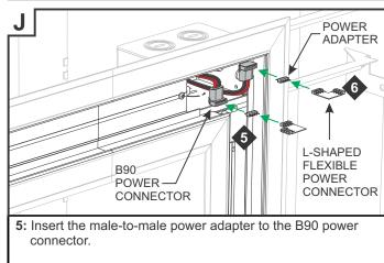
6: Connect the L-Shaped Flexible Power Connector to the male-to-male power adapter.
