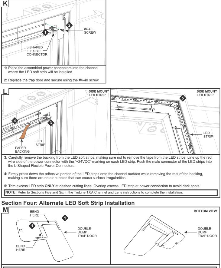
NOTE: For installations where the LED Soft Strip will lay in the bottom of the channel it is necessary to use a double-dump trap door.
