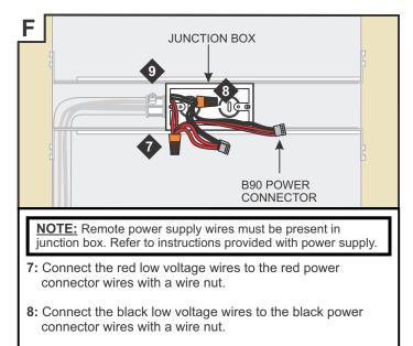
9: Place all wire nut connections inside the junction box.
