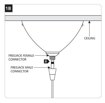
8 Screw the Fixture FreeJack male connector into the FreeJack female connector.
