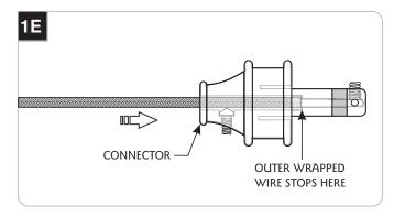
Feed and push the coaxial cable into the connector. The coaxial cable will come to a stop point after being inserted 3/4" into the connector.
