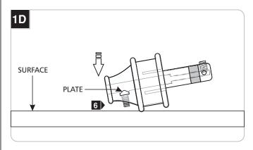
Tap the connector on a hard surface with the set screw facing down, so the plate inside drops into place.
