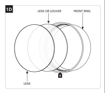
4 Place one or at most two lenses and/or louver into the front ring.
