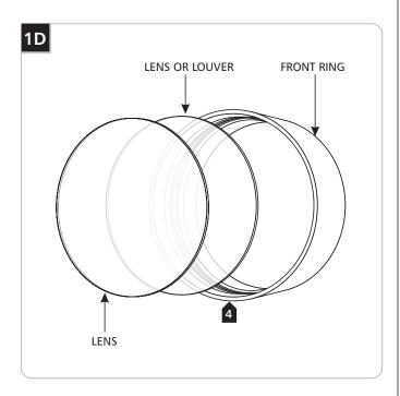
4 Place one or at most two lenses and/or louver into the front ring.
