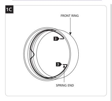
3 Squeeze the spring ends and remove it from the front ring.
