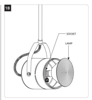
Use 120 Volt, 39 Watt Ceramic Metal Halide PAR20 Lamp.
