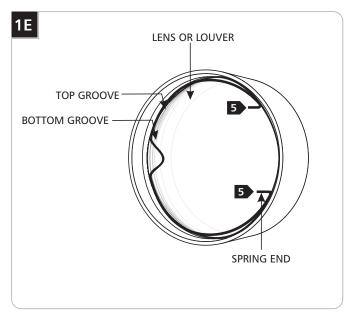
Squeeze the spring ends and place on top of the lenses (louver) and into the top groove of the front ring. Use the bottom groove if a single lens or louver is used.
