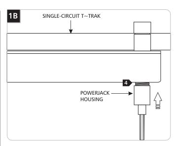
**NOTE:** Use **MAX 35** watt fluorescent fixture with the Single-Circuit T~trak compact fluorescent adapter.
