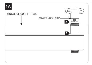
**NOTE:** Turn off power to Single-Circuit T~trak before installing the compact fluorescent adapter.
