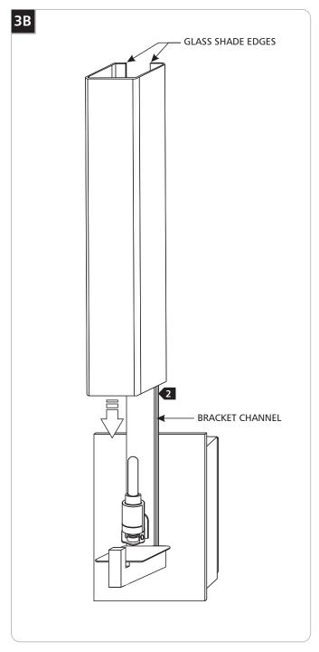
2 From top of the sconce carefully slide the glass shade edges into the bracket channels.
