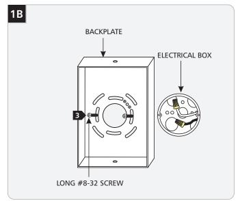
Mount the backplate to the electrical box with two long #8-32 screws.
