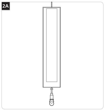
1 Gently lift both the glass shades up to expose the socket.
