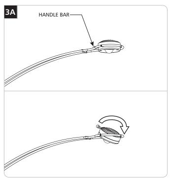
**CAUTION:** Fixture will be hot. Do not touch any other surface of the fixture. Only use handle bar to tilt the lamp and change light direction.
