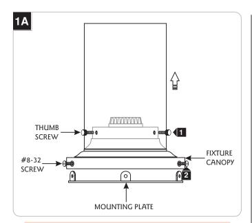
**NOTE:** It is recommended to remove the glass shade from the fixture base to avoid breaking it during the installation.
