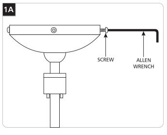
Separate the crossbar from the canopy by removing all four screws with the Allen wrench provided.
