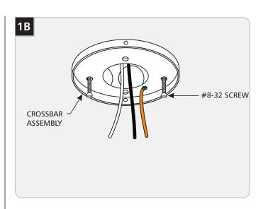
Mount the crossbar to the electrical box with the two #8-32 screws provided.
