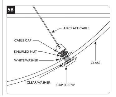
From outside of the glass, insert the cap screw with a washer through one hole.
