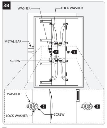
2 Mount the pan to the metal bar with the washers, lock washers and screws provided.
