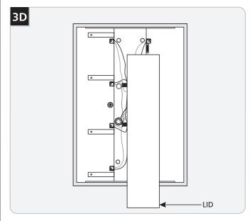
6 Replace the lid onto the center housing and tighten the screws.
