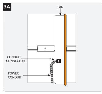
1 Connect the power line conduit to the connector.
