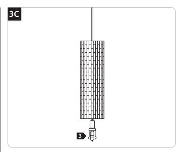
For incandescent versions, use MAX 50 Watt Bi-Pin Halogen Lamp.
