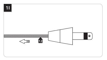
12 Pull the coaxial cable toward the fixture to smooth the wrinkles.
