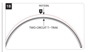
4 Constantly check the curved Two-Circuit T~trak against the pattern.
